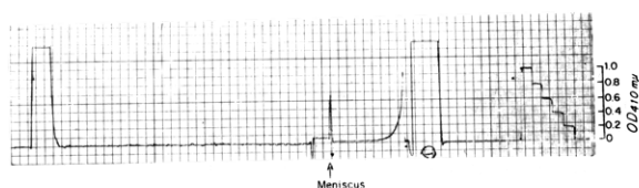
FIGURE 4: High-speed sedimentation equilibrium patterns of hydroxylamine oxidase. The trace was recorded with light of wavelength 410 m\mu after 15 hr of centrifugation at 14,000 rpm. Solvent, 0.1 M Tris-HCl, pH 7.3; protein concentration, 20 \mu\text{g}/\text{ml} . For illustration purposes, a medium scan speed was used.
